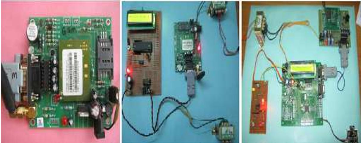
1. ZIGBEE-GSM BASED AUTOMATIC METER READING SYSTEM
